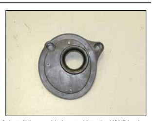
6. Install the provided venturi into the K&N® back plate as shown.
