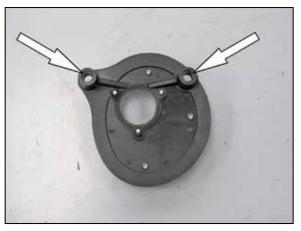
9. Install two of the supplied O-rings onto the back side of the back plate.
