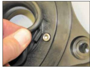
7. Install the three throttle body bolts supplied though the holes in the back plate and venturi.
