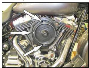
13. Install the K&N® air filter onto the back plate and secure with the provided hardware.
