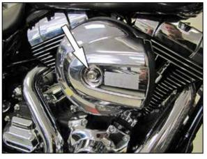
3. Remove the bolt that secures the bonnet to the air filter and then remove the bonnet.
