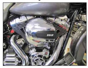
14. Install the factory bonnet onto the air filter and secure with the factory bolt. Install the decorative badge onto the bonnet.
