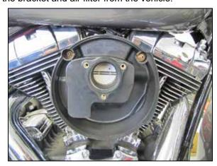
5. Remove the two breather bolts that secure the filter base to the engine and then remove the filter base from the engine.
