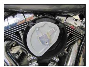
4. Remove the three bolts that secure the bonnet mounting bracket and air filter, and then remove the bracket and air filter from the vehicle.
